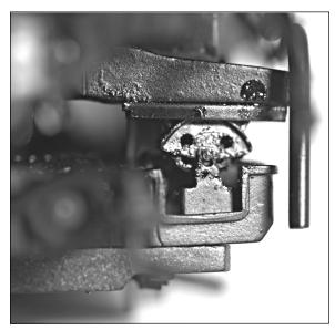
The photo to the left illustrates the correct setup for the rocker units, notice that the rocker head is centered over the base unit, this will allow free movement in either direction.
